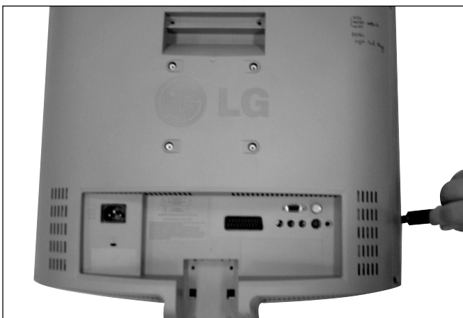
#5 Open the Backcover's latch with jig
